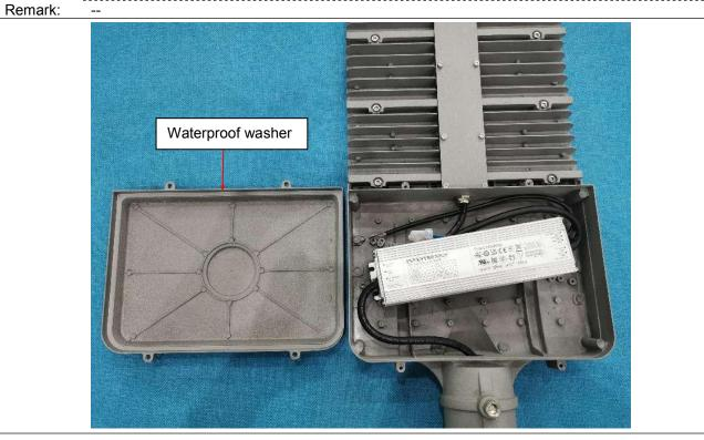
Details of: LED driver view for model SZG510-250W
